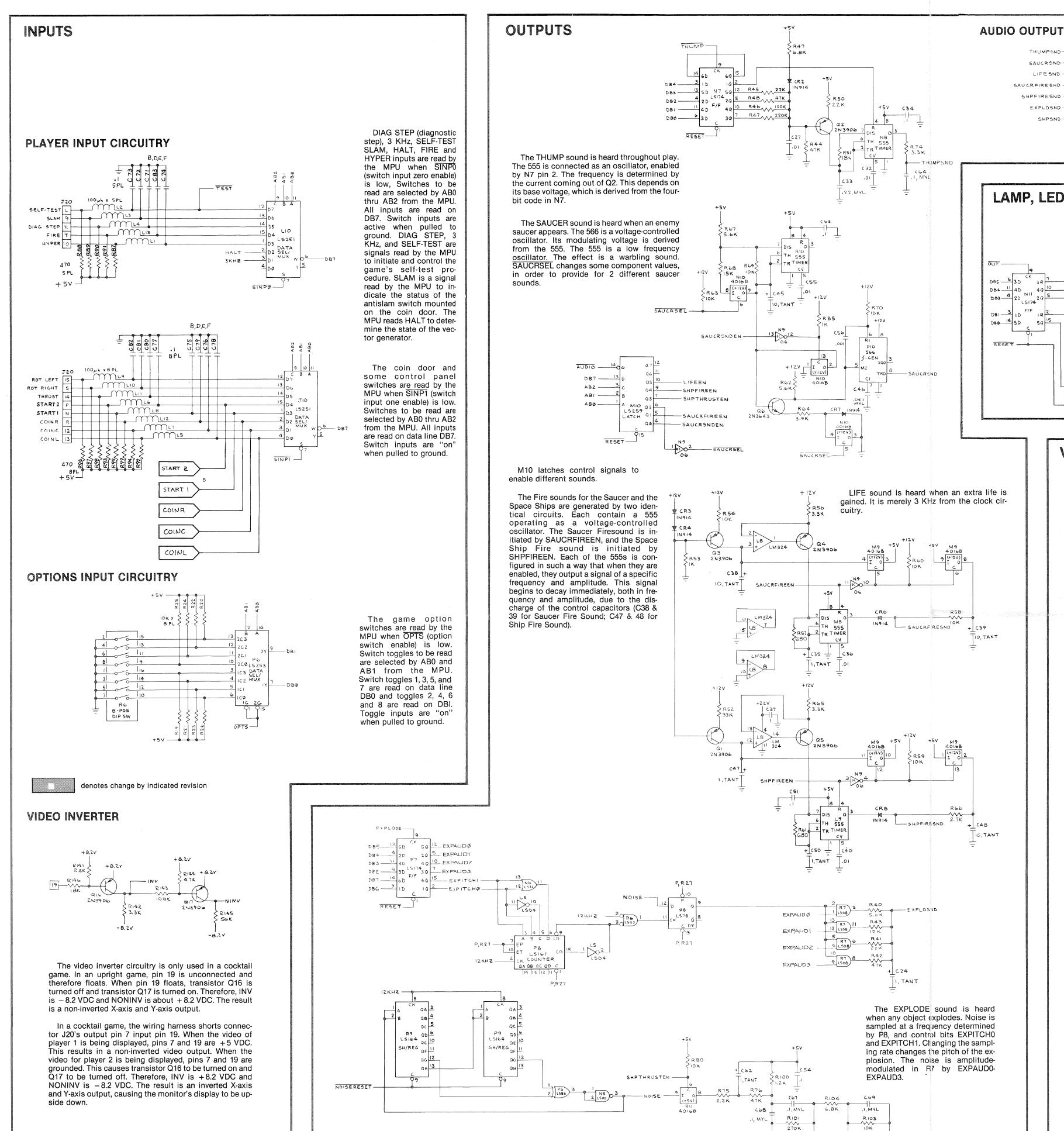
R9 and P9 generate random noise. This noise is filtered by P11 and produces the rumble sound heard when the ship is
