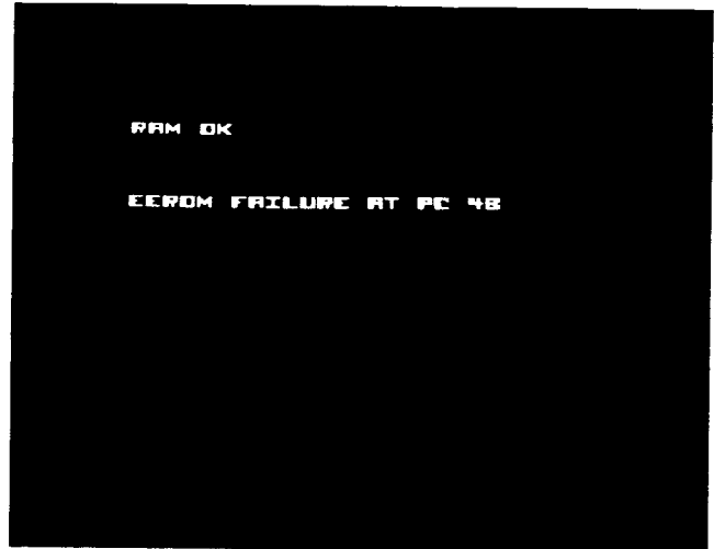
Figure 2-2 EEROM Failure Video Display
