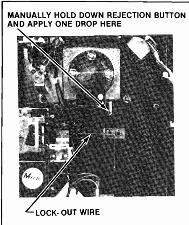
Figure 4-6 Close-Up View of Lubrication Point
