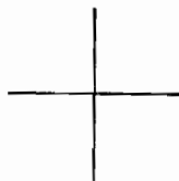
LINES ARE NOT CONNECTED
