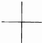
LINES ARE NOT CONNECTED
