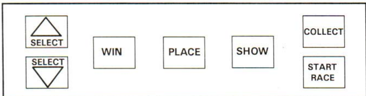
CONTROL PANEL WITH COLLECT BUTTON (Ticket dispenser installed)
