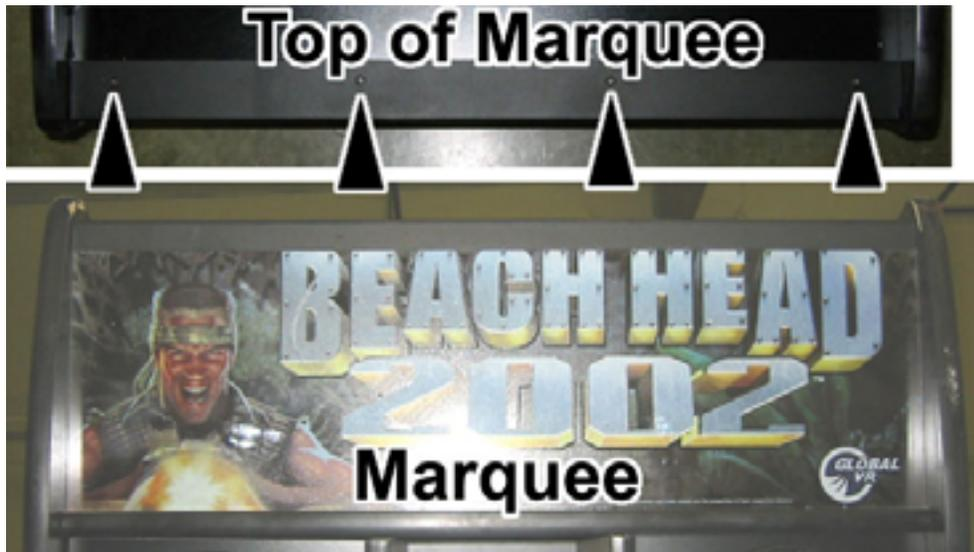
Install the new Marquee artwork by removing the 4 T-25 security Torx screws across the top retaining bar that hold the Plexiglas and Marquee as shown by the arrows in the picture above.
