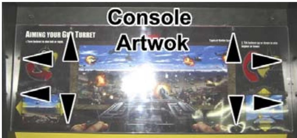
Install the new Console artwork by removing the 6 T-25 security Torx screws around the console that hold the Plexiglas and Console artwork as shown by the arrows in the picture above.
