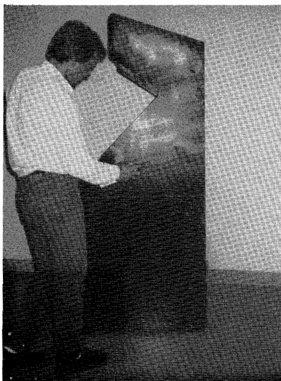
Spray the side of the cabinet with glass cleaner, this will allow you to align the side decal before it adheres to the cabinet.
