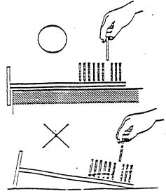
Note: Lay PC3 flat on table with 079 Shield Cover hanging off table as shown.
