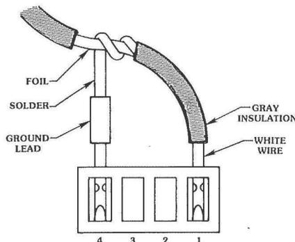
Be careful not to strip away the foil underneath. Make a small jumper
