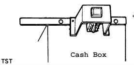
The service switch is used for adjustment. When this switch is depressed, game can be played while the game counter does not work.
