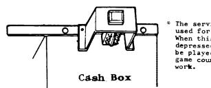
\* The service switch is used for adjustment. When this switch is depressed, game can be played while the game counter does not work.
