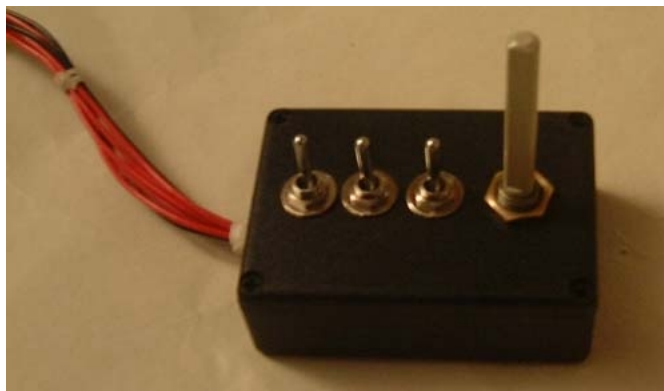
The Control Box Built and Wired Up
