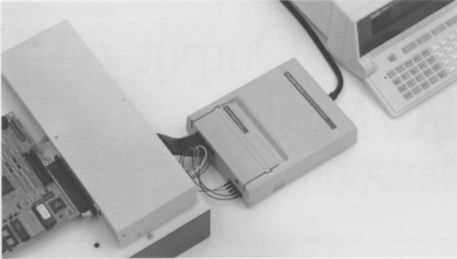
Vector Output I/O Module Connected to a Card Edge Fixture and the 9100A.
