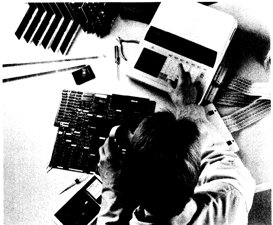
The Fluke 900 isolates the functional board failure to the failing component. It captures dynamic and intermittent malfunctions as well as static component failures.
