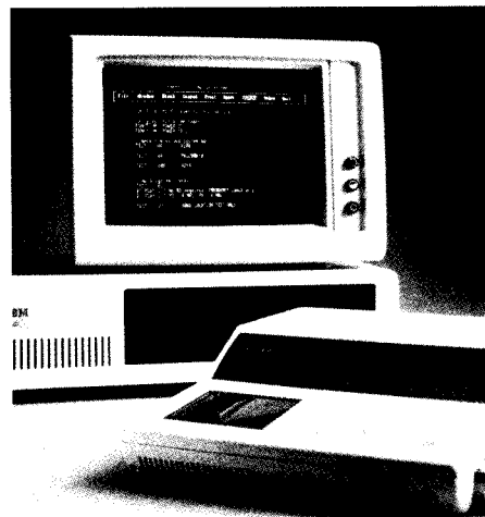
The 900 provides the ability to exchange files with a (personal) computer via its standard RS-232C port. A Test Sequence may be uploaded to facilitate editing and to add operator instructions as well as comments.
