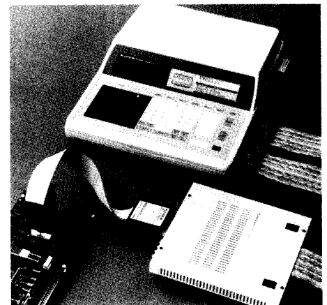
The interface buffer is connected to the mainframe via a four-foot ribbon cable. A full set of clips is available to accommodate DIP style as well as surface mount small-outline-style digital components.
